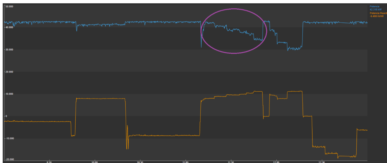
Figure 7 Active (blue) and reactive power (orange) generated at local test on 26/05/2021
