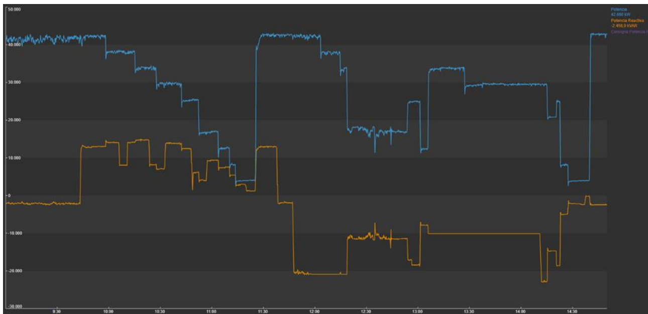
Figure 9 Active (blue) and reactive power (orange) generated at local test on 08/06/2021
